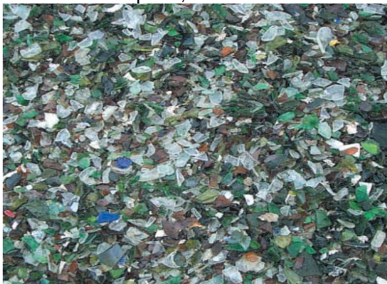
Figure 2: Mixed coloured glass called cullet, Alex Fraser Asphalt, Laverton
